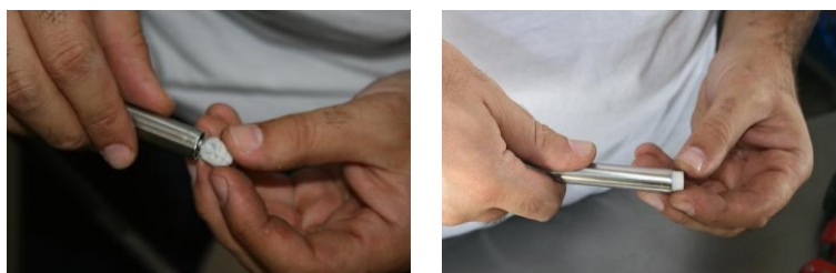
Figure 12: End Plug placement
